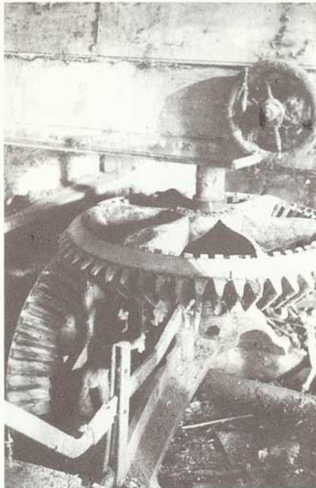
Plate VI Branston barn. The drive gear to the Peak stones. Catherine M. Wilson.
